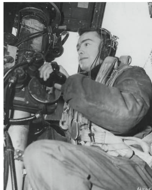
Sgt Jim Wise, 13th Bomb Squadron peers through the periscope that the gunners used to sight in the enemy.
