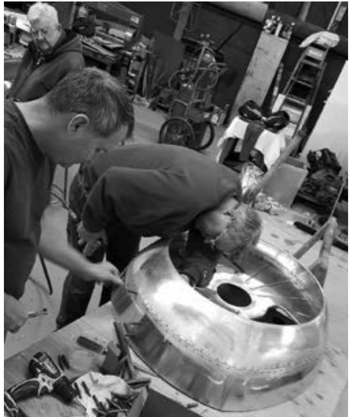
Paul Dougherty and Rob Waring transform metal plate into a SPAD cowling. The curved shape was formed by hammering and hand working on an English wheel. A liberal amount of colorful language was employed to complete the shaping. Paul Dougherty Sr. stands watch.
