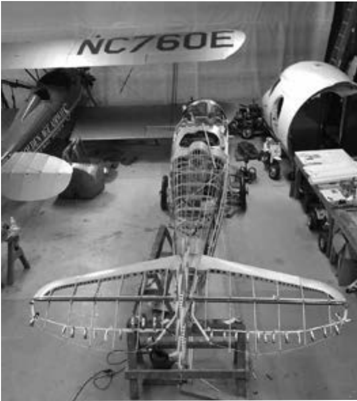
The SPAD, minus its wings in the GAAM shop. The elevator rear spar is being glued together.
