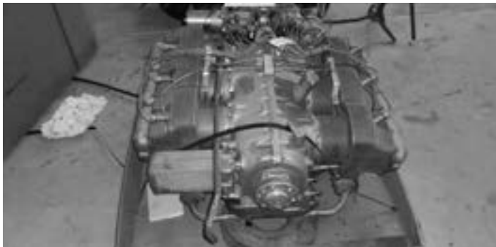
The Continental O-470 motor which will power the GAAM SPAD was originally in a Cessna 182. One of the challenges to re-engining the airplane was fitting this modern engine into the profile originally occupied by a V-8 220 HP Hispano-Suiza engine.
