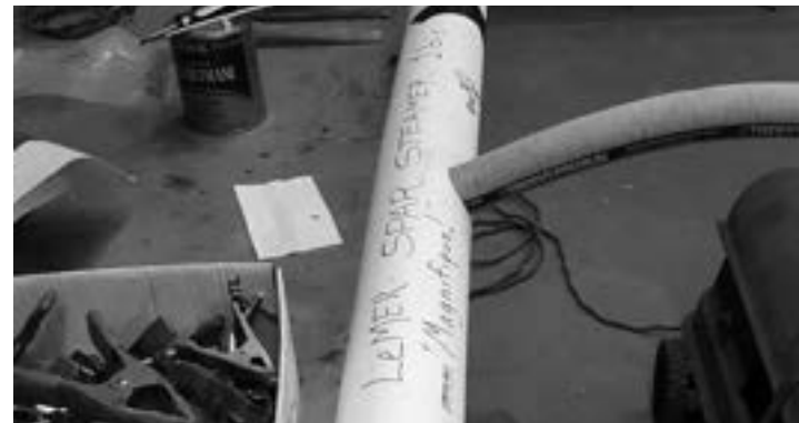
The upper wings spars needed to be steam straightened. The improvised "Pierre Le Mer Spar Steamer" consists of a PVC tube and sealed bucket of water connected to the PVC by a rubber tube and a kerosene heater. The improvised steamer proved successful.
