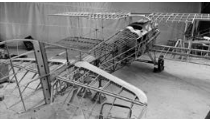
Rear view of the assembled SPAD. The blue elevator spar reflects the WWI French practice of painting metal parts and fittings blue.
