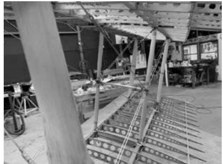
The details of the wings are evident in this photo. The interplane struts are actually steel tubes which are covered with aerodynamic spruce fairings. The many brace wires were also individually sized and their ends hand formed and soldered.
