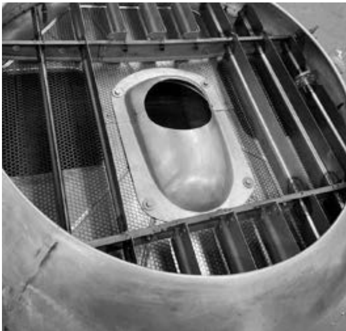
While the original SPAD had a water-cooled engine, the GAAM machine is air-cooled. To maintain the illusion of a radiator with operable cooling louvers, the SPAD had a faux-radiator and the louvers, though they appear to be operable, are actually welded fixed in place. The small pulley at the far right was added, though completely inoperable, to complete the illusion.
