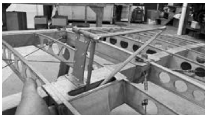
The aileron bellcrank assembly. This connected to a rod which runs vertically to actuate the ailerons on the upper wing. Two were required and of course, there is a left and right-handed version
