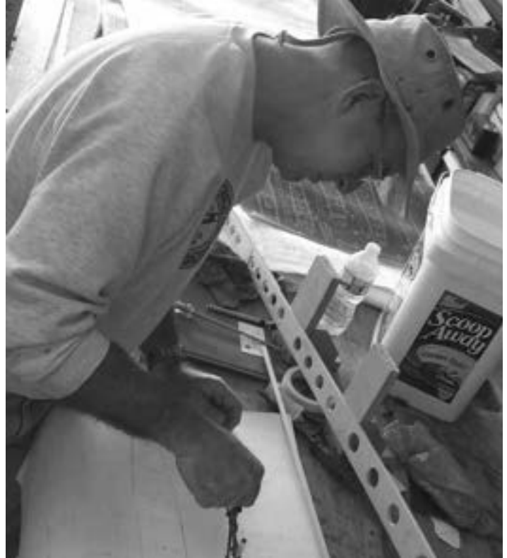
Museum director Gerry Wild lofts ribs for the horizontal tail. All of the individual components were drafted, hand cut and then fitted to form each component of the airplane. The process was repeated for the horizontal and vertical tails, wings and many individual fuselage components.
