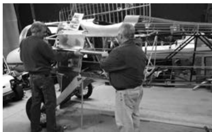
One of the defining characteristics of the SPAD is the metal work from the cockpit forward. Here museum President Paul Dougherty and museum director Mike Cilurso are fitting the long exhaust pipes which are a SPAD hallmark.
