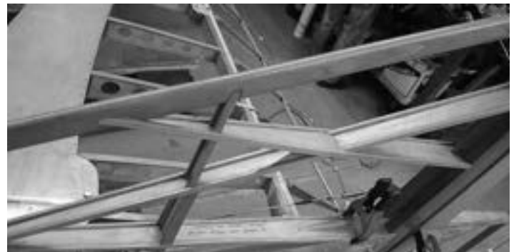
The vertical fin is a jigsaw puzzle of individual pieces – this component is composed of no fewer than 28 individual pieces.
