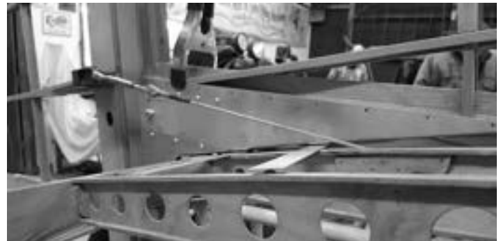
Details like this metal fitting with a small, sliding inspection door, are among the numerous details that make the replica look like the original airplane.
