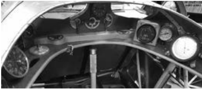
The SPAD cockpit under construction. Unlike modern airplanes, the SPAD cockpit looked like a random assembly of instruments. The tachometer – seen on a tilt at left, the clock in the center of the dashboard, and the leather rimmed altimeter at the far right – are all original 100 year old instruments.
