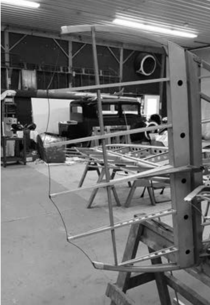
The trailing edges of all flight surfaces are formed with wire. The small, copper clips which secure the wire to the wooden structure are wrapped with fabric to prevent chafing.
