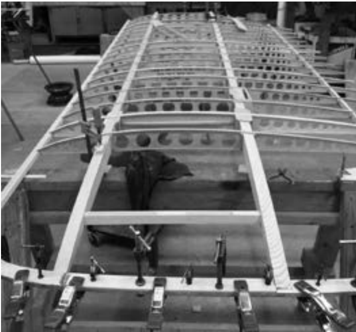
Most wing ribs could be constructed before installation. The wing tips were the exception, requiring the volunteers to build them in place. Similarly, the wing tip bow was patterned, but installed in place and sanded to the proper profile by hand.
