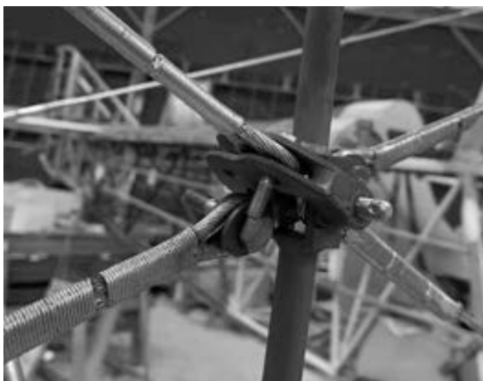
A prime example of the (mostly unnecessary) complicated design of this airplane. This detail is the mid-wing interplane struts, here without the aerodynamic spruce fairings. The wire bracing and complicated fittings replicate the original design exactly.
