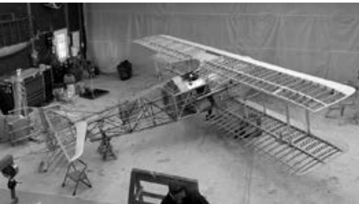
The SPAD assembled – minus its ailerons – in the GAAM shop. The airplane is assembled and disassembled multiple times during the construction process to ensure accurate fit.
