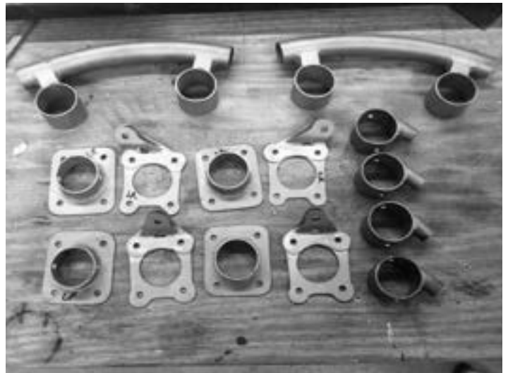
Metal landing gear components – all fabricated by volunteers – made to original specifications. Transferring these designs from the original prints to patterns to completed component requires extreme attention to detail. Any component not precisely to size was rejected.
