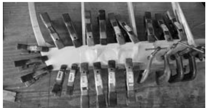
“Just like a big airplane model”. Waxed paper is used to keep the clamps from sticking to glued joints. This is the rudder leading edge.
